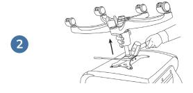
With one hand grab the gas lift and try lifting it upwards while hammering the mechanism with the other hand. Continue to do this until the gas lift is free.
