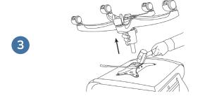
The mechanism is now free and can be replaced. Now you can undertake further repairs such as changing the gas lift.
