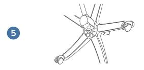
Hammer between the gas lift and the hole until the gas lift loses and becomes free.
