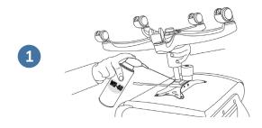
Turn the chair upside down. We recommend that you first place a towel on the floor to prevent possible spills of the WD-40 liquid. Aim the nozzle of WD-40 in the mechanism and spray it.
