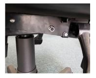
3 Using an adjustable spanner, turn the nut ¼ of a turn clockwise. 3 Check the seat tilt no longer slips. If it still doesn't hold position, repeat the above step another quarter of a turn, until the clutch holds.
